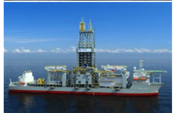
Atwood Achiever: new build 6 th generation ultradeepwater 3,650m WD drillship
